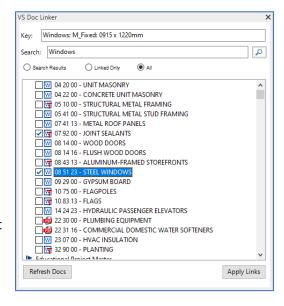
Note: The above model key links are from model elements to the required spec(s) which provide a good level of coordination. VisiSpecs also supports linking the same elements directly to the spec paragraphs and bracket options for advanced doc automation and coordination. The advanced linking is typically implemented after the initial spec section linking. Refer to the VisiWord Tutorial on Model Key Filtering.
